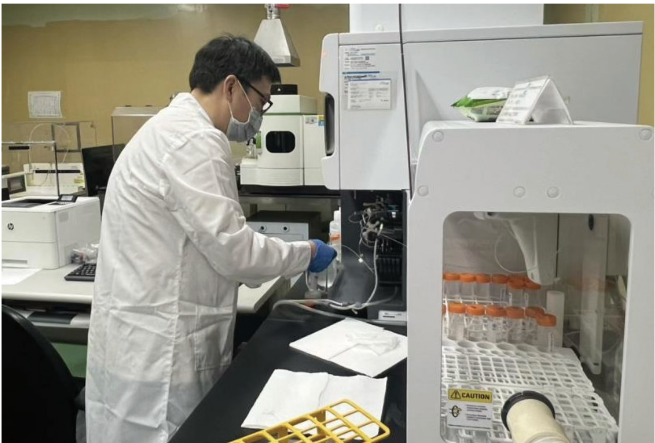
■ NERI staff operating an inductively coupled plasma optical emission spectrometer (ICP-OES) (2)
