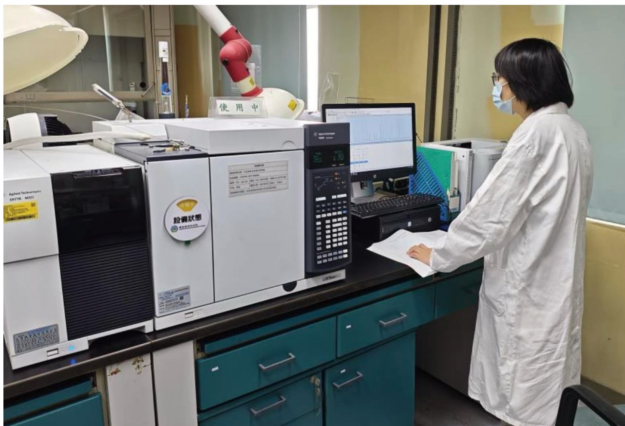
■ NERI staff operating a gas chromatography-mass spectrometry (GC-MS) instrument
