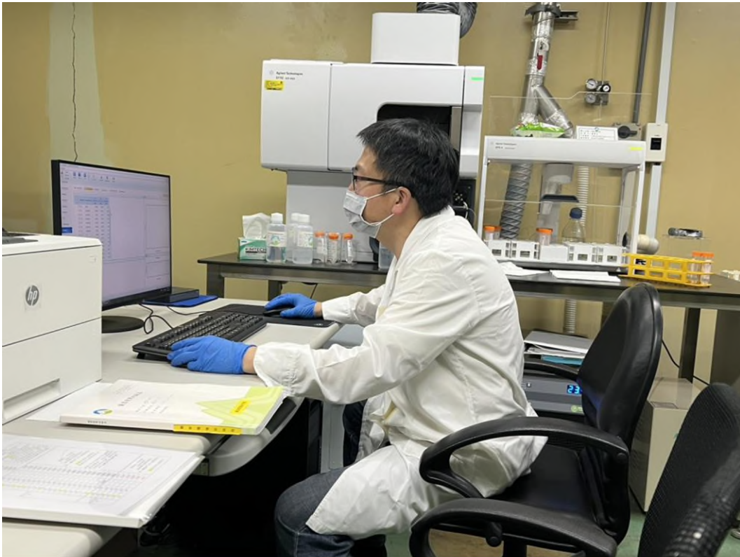
NERI staff operating an inductively coupled plasma optical emission spectrometer (ICP-OES) (1)
