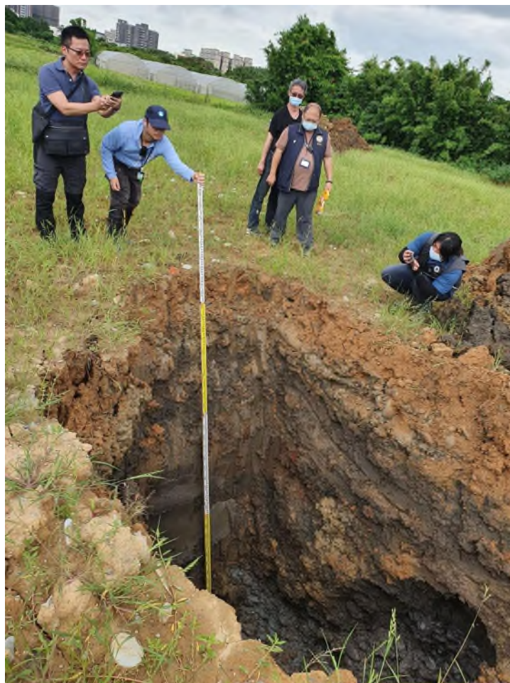
Taking a measurement of backfilling depth.
