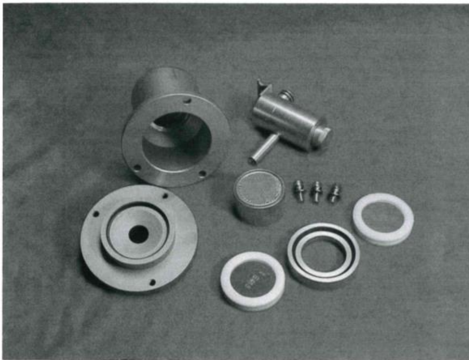
Figure 1.4 Photograph of the disassembled SASS Canister, showing the SCC Inlet, the MgO denuder, the front and back filters and the protective canister.
