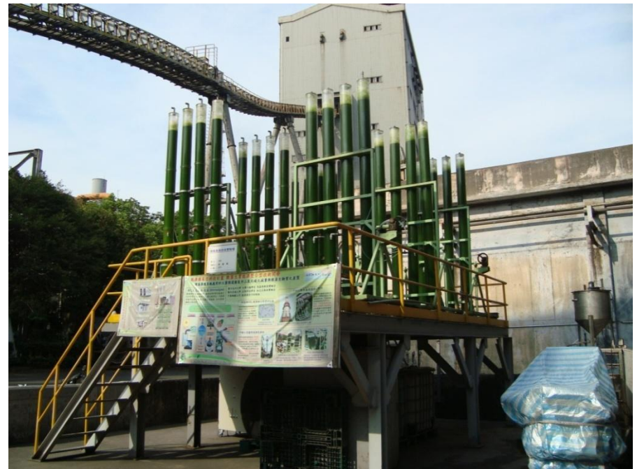
Cultured volume: 40 L/reactor (Total: 6 x 40 = 240 L)
